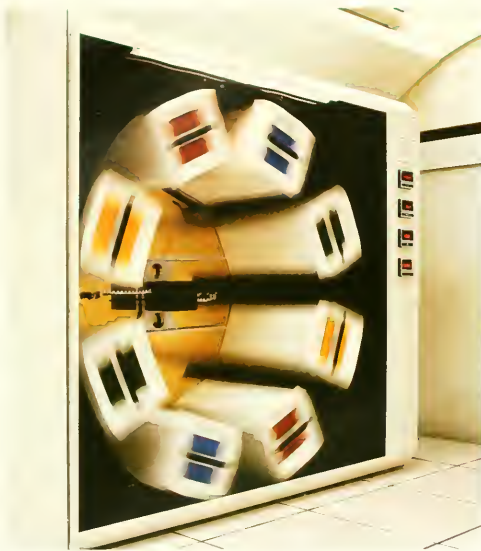
This mockup of a 1.8-meter centrifuge is undergoing tests at NASA's Marshall Space Flight Center. The centrifuge was designed at Ames Research Center for use on the Space Station.
